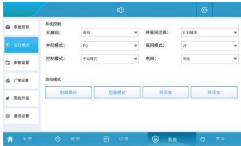
Figure 5.19 Manual and off-grid switching mode setting interface
