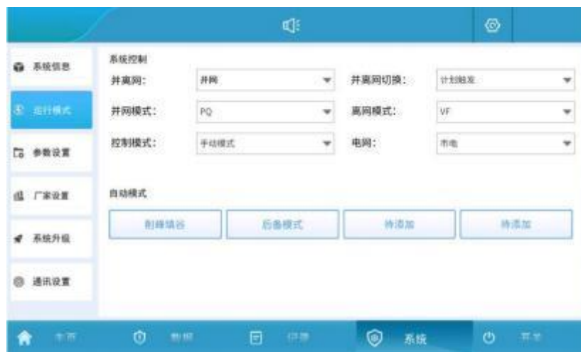
Figure 5.9 _ Grid-connected manual mode setting
