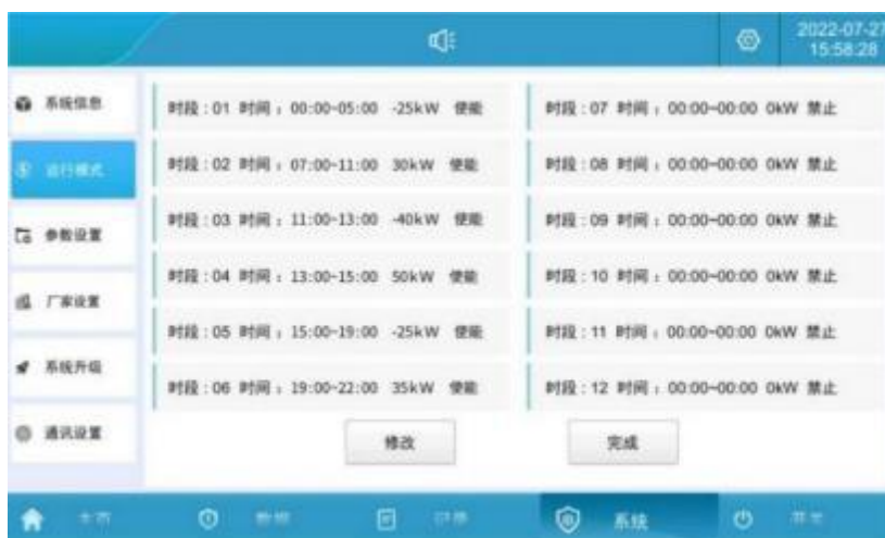
Figure 5. 13 Peak shaving and valley filling charging and discharging setting interface
